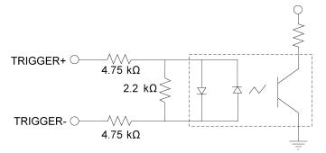
28VDC Max. Across input pins - Transition approx. 8VDC (Nom.)
