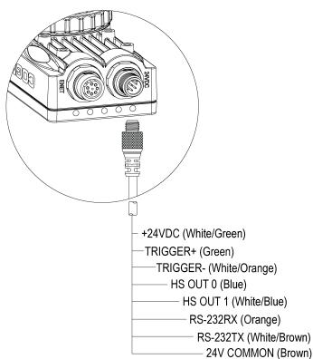
5. Restore power to the 24VDC power supply and turn it on if necessary.
